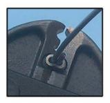
The sleeve should be squeezed into a cylinder shape. (Do not split the sleeve into an "8" shape.) The one wire should be pushed tight against the other wire.
