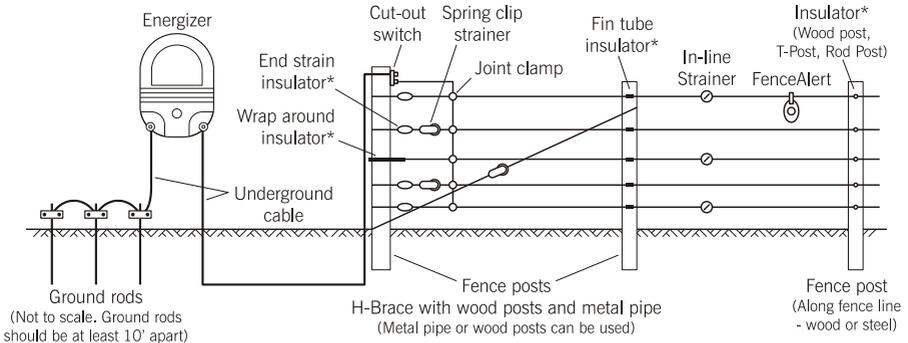
\* A single type of insulator can be used on the fence line or a mixture of each depending on individual needs and post type.
