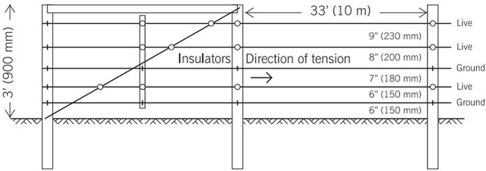
H-Brace – Very simple to erect and most suitable as a high tension strainer, excellent in areas where the soil gets very wet or where heavy frost occurs.
