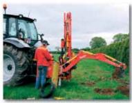
When the digging arm is not in use ensure the safety bars are in place and the shut off valve is in the locked position.
