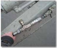
Once the postdriver has been securley fitted to the excavator the support leg can be removed and the hydraulics connected
