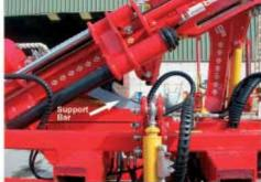
If your post driver has been folded for transport it must be assembled prior to use by removing the support bar and putting the mast tilt ram into position.
