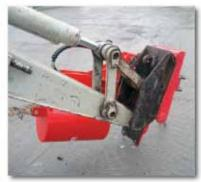
Before attatching the postdriver to your excavator you must first check that all pins and hitch dimensions are correct, Bad or loose fitting hitches can fall causing damage or injury.
