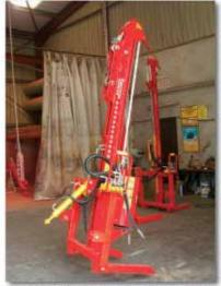
Rear mounted machines are lifted using a crane or hoist using a chain connected to a lifting pin on the mast and it is the responsibility of the person lifting the machine to ensure the chain is the correct strength to lift the Post Driver.
