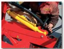
Replace both pins and secure with nuts before carefully removing chain,
