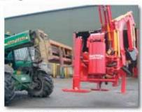
Side mounted machines are loaded via a forklift using the back shift slides. Carefull attention must be paid when lifting machines as weight distribution may not be central to where the forks are lifting from. Machines are only lifted for loading/unloading and are not to be transported for any distance in this way.
