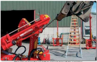
When pins are loose they can both be removed along with the support bar.
