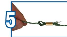
Fold other end over the first crimp, overlapping both sections. Crimp again so the twine is secure.
